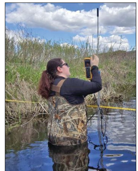
Jaxsyn Olson collects a stream sample using a Van Dorn (top). Julia McGee uses a FlowTracker for a streamflow measurement (bottom).
